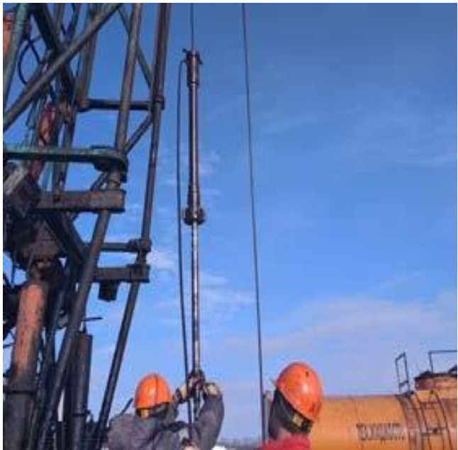
Run of the ultrasound device into a hole
