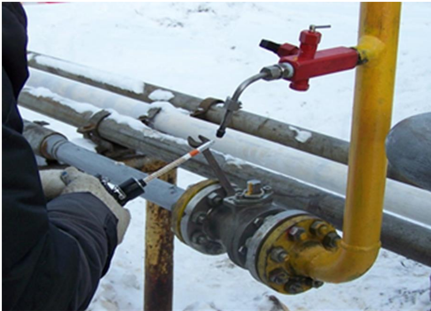
Photo of express analysis with indicator tubes
