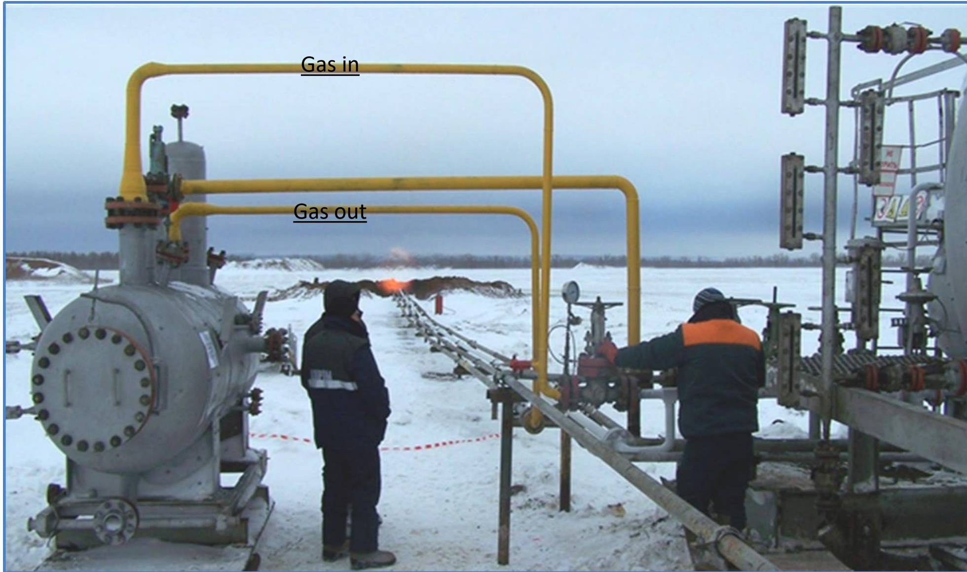
Photo of the field trials of Ecoil series scavenger for gas treatment at the Orenburg oil and gas condensate field.
